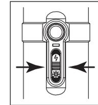
Turn on the LED Flashlight by pushing the ON/OFF switch to center position.
